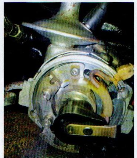
A very late North American market MGB with a Lucas Constant Energy electronic distributor (the good one).
