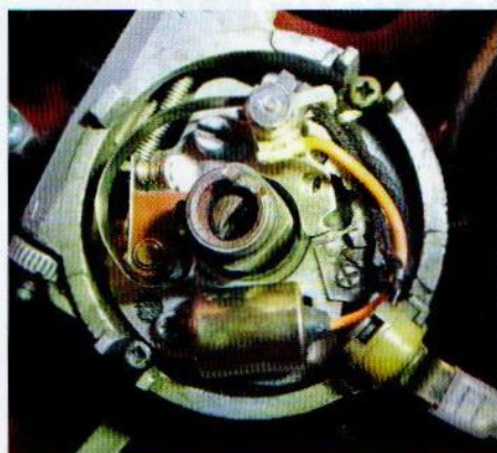
This is a typical Lucas 25D4 points distributor, with the arrow indicating the direction of rotation.
