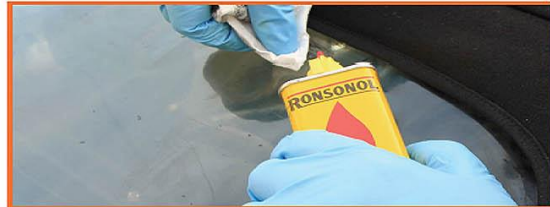
Ronseal, the car enthusiast's special weapon is an essential addition to your kit, with a multitude of uses. I used it on our plastic window to get rid of the black splashes. It made a difficult job very easy...
