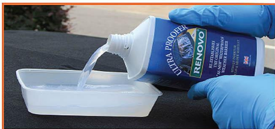
With the soft top looking nicely black and feeling revived to touch, the final step is the application of Renovo's Ultra Proofer, which helps make the material remain resistant to water. Again we went the extra mile and applied three coats. After the first one the liquid began to bead on the surface showing that it was working. This stuff smells like PVA glue without the stickiness.
