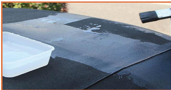
As you can see, Ultra Proofer goes on nicely with a 2in brush and once again we divide the hood into sections for easy application.
