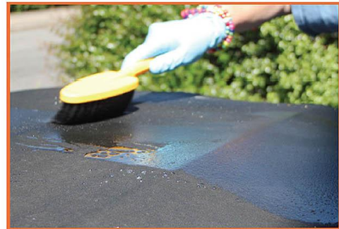
First step was to brush any loose dirt and bird lime away, while also washing it with clean, cold water. The day we chose to do our test wasn't ideal as the temperature was in the low eighties.
