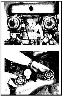
clearance between screw and stop - making sure that the choke fast idle is not impeding the return of the throttle spindle. Screw in both idle screws by an equal amount starting around 1½ turns each and then start the engine. Adjust the screws again evenly until an acceptable tickover is reached.
