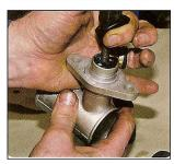
**8. PISTON IN:-** pressing in the piston with the pushrod, refit the cir-clip. Use a bench vice to hold the unit if preferred, but mind your new paint finish. Now fit the gaiter. Job done.
