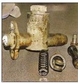
**2. TAP IT OUT:-** *Tap the cylinder on a wooden surface to allow the piston to protrude enough for its removal. Its return spring will drop out freely.*
