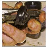
6. FIT GAITER:- The new rubber gaiter can be more easily fitted using long-nose pliers to carefully stretch it over the pushrod washer.
