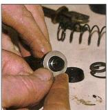
4. NEW SEAL:- Fit the new piston seal and any shim washers, such as the one seen here, using plenty of brake fluid as lubricant.
