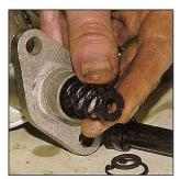
**5. SPRING LOADED:-** *Refit the spring, followed by the rebuilt piston. Again, use plenty of brake fluid to lubricate the seals.*
