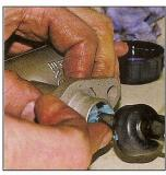
7. GREASE IT UP:- Use plenty of rubber friendly grease, (Corrosion Block) to lubricate the pushrod in the piston end cup.
