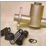
**3. CLOSE INSPECTION:-** Thoroughly inspect the bore and piston for any damage or terminal wear. Bin (recycle) the lot if you find any excessive wear. Stuff tissue into the cylinder bore. Prepare and paint the whole unit.
