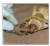
**1. REMOVE PUSHROD:-** Using cir-clip pliers, undo the cir-clip and remove the pushrod and its rubber gaiter.
