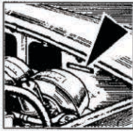
The Body Number for early chrome-bumpered cars is stamped on a plate on the left front valance behind the radiator diaphragm as illustrated, or in some cases, in front of the radiator diaphragm.
