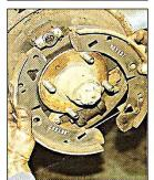
2. SHOES OFF:- Unclip the top spring, then lever the shoes out of contact with the cylinder and hand-brake mechanism. Note which way round they are, drum should pass over the lining free section last when moving forwards.
