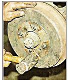
1. REMOVE DRUM:- Spray brake adjuster nut on the back with oil and back them off as far as possible to make drum remove easier. If still tight, try tapping drum onto the axle with a soft-faced mallet. This should jolt it free.
