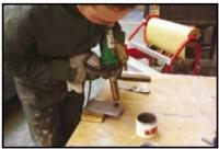
**4.** The C-post repair is tricky in that it is a vertical panel and it is easy to end up with a large gob of lead on the floor and very little on the panel. Therefore, first practice on a horizontal piece of scrap metal to get a feel for how the torch (or in this case a plastic welder hot air gun) imparts its heat.
