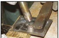
**5.** The gentle heat of the hot air gun means the process is slow, but also very controllable. With the panel tinned and loaded with lead (see steps 6-9), you can see when the metal is starting to go pasty and catch it easily with a wooden paddle to spread around the work area before it goes liquid.
