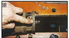
As the unit is re-assembled, ensure that the pip on each end plate engages fully with corresponding cut-out in the motor's casing. Don't force the end plates home if they won't easily locate, investigate/try again.
