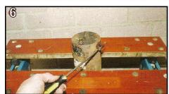
Unscrew the unit's end-cover, released carefully ease the cover off the motor's body. This exposes the apertures in the casing through which the brush gear can be examined and reached.
