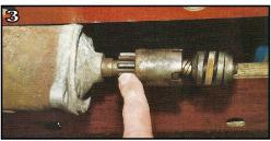
Check teeth on the main drive pinion, they should have clear-cut profiles. If they are severely worn, you will need to replace. (special tool needed)
