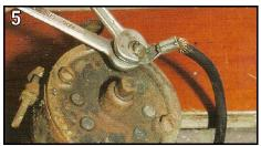
Remove the power lead from the main terminal on the motor. Use a 7/16in AF open-ended spanner to hold steady the inner nut on the pillar, while releasing the outer nut (also a 7/16in AF)
