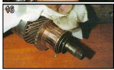
Gently clean the commutator, using a cloth moistened in petrol. If necessary apply a little fine glass paper to remove minor burning marks. Do not use emery cloth because the particles will cause damage.
