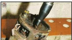
Loosen the two long through-screws running the length of the starter motor. These are often very tight, so apply some penetrating oil in advance and then use a good sturdy screwdriver to release them.
