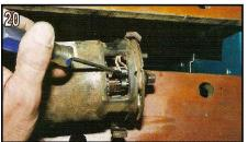
As the end plate is guided home, hook the pressure springs for each of the end plate brushes into their correct positions - acting in the centre of each brush (*between the two copper braids attached to the brush*)
