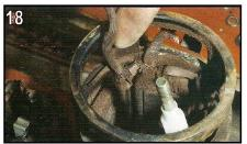
The brushes attached to the field coils are secured via flexible cables. To replace the brushes, these wires need to be cut and the cables of the replacements soldered to them.
