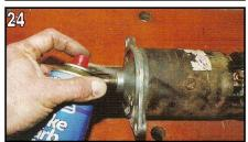
Use carburettor-cleaner spray to spruce up the aluminium end plate adjacent to the Bendix drive gear. Leave final preparation for repainting until the unit is re-assembled. (*to avoid internal contamination*)
