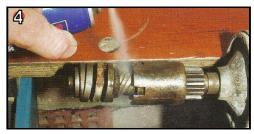
Pull back the drive pinion/barrel assembly and ensure that it returns easily on its own. A spray lubricant can free up sticky unit, but don't use oil, attracts dirt which in turn clogs up the mechanism.
