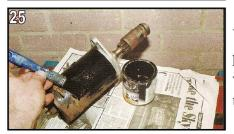
With the unit's casing lightly rubbed down using fine wet/dry paper, employed dry, and having wiped the surface with a spirit wipe solution *(to remove dust)*, we applied black engine lacquer to finish off the job.
