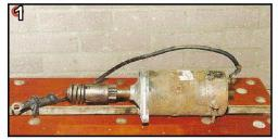
The starter motor as it came off the MG. It's physical condition beneath the dirt appeared to be really quite good, even if it is running slow.
