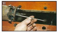
Make sure that the motor is horizontal before finally releasing and pulling out the two through-screws. (otherwise the motor may come apart and its components will land on the floor, causing damage and swearing!)
