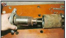
Extricate the commutator/armature assembly, taking great care not to damage this, nor the comparatively delicate field coils within the casing, as the commutator/ armature assembly is removed.
